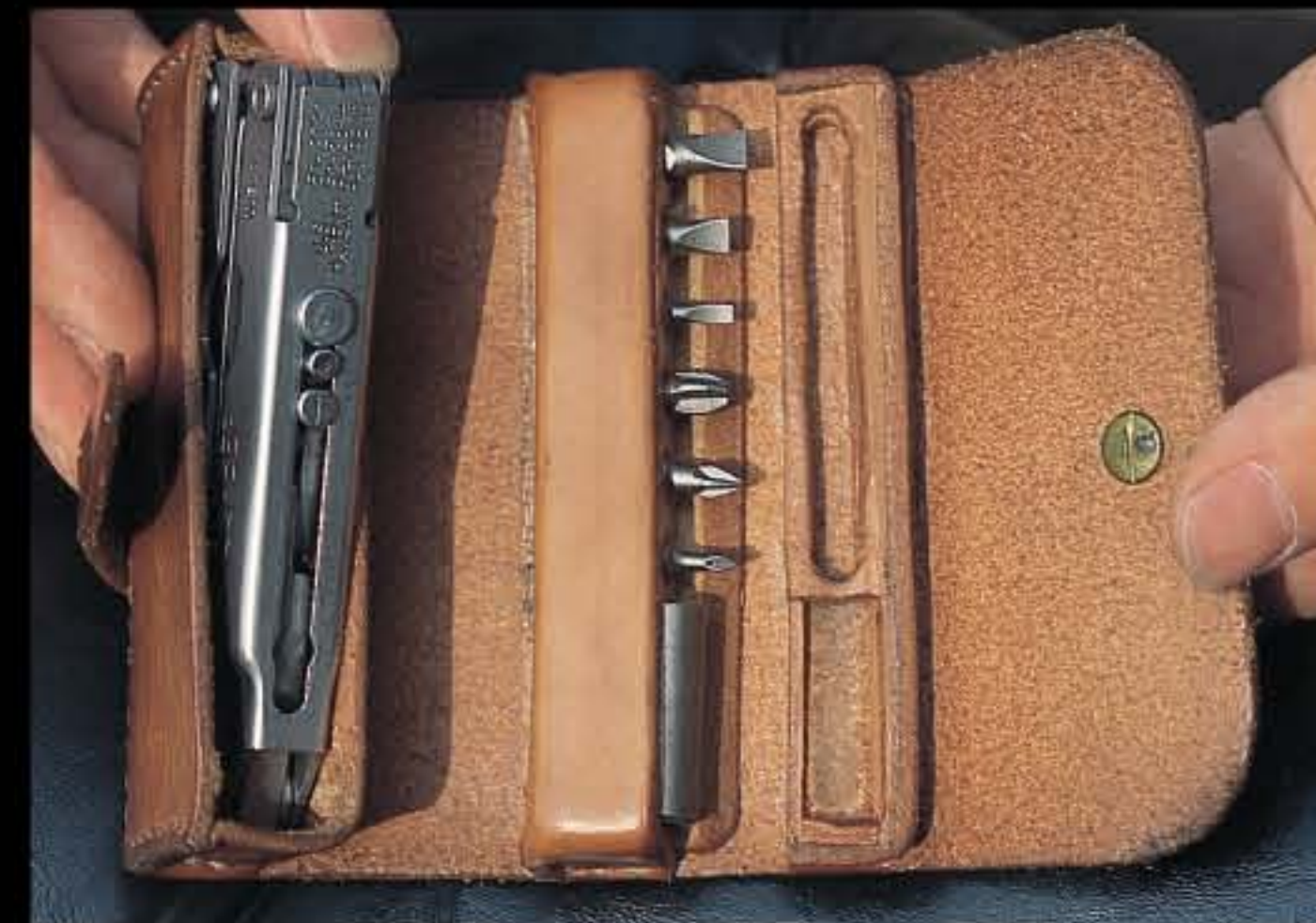
As you can see, when the catch is released, the weight of the pliers flips them out ready for action.
